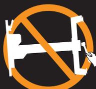
**Cart Must Remain Upright! Tipping Cart On Side May Cause the Work Surface to Disengage Causing Serious Personal Injury and Property Damage.**
