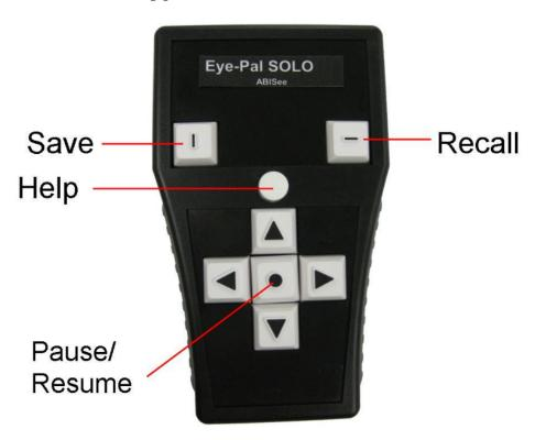
**Help Button** –located in the middle of the keypad, above the Up Arrow, it is a white round button. It will say the function of each button on the keypad. Hold down the Help button and any other button on the keypad at the same time. You will hear a description of that button and its function.
